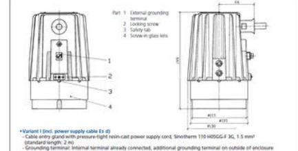
Dimensions for Lumistar luminaires ASL 55-LED and ESL 55-LED
